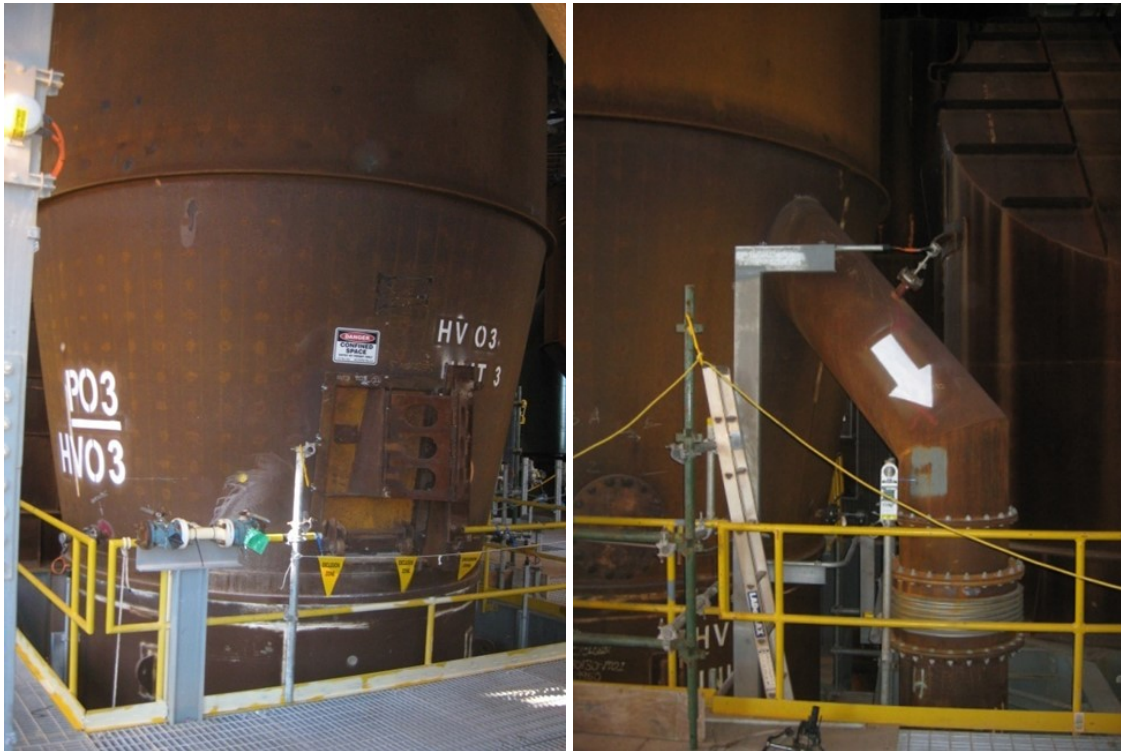
Figure 9. Holding vessel body (left) and material discharge to CO1 at 900 Deg C (right).
